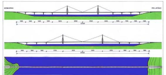
*Fig. 2*: Options of combined crossing to Pelješac: cable-stayed bridge in the middle and approaching bridges as continuous hollow box girder of varying height, with middle span of the CSB 500 m (up) and 650 m (below).
