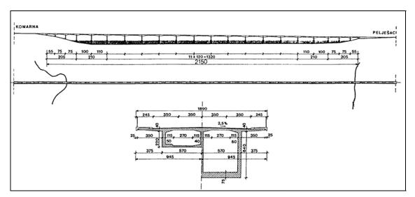
**Fig. 1** An option of the crossing with spans at max. 120 m and a low grade line, with free cantilever construction on columns or combined with precast 50 m long girders in the center of the field.
