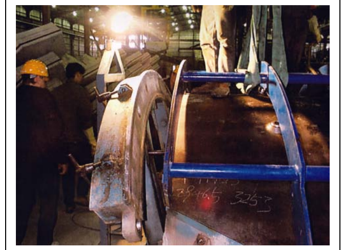
Figure 7. Calibration of steel mould by steel calibration device..
