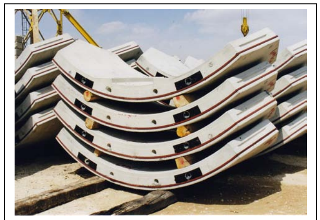
Figure 8. Segments on the storage near to production hall.
