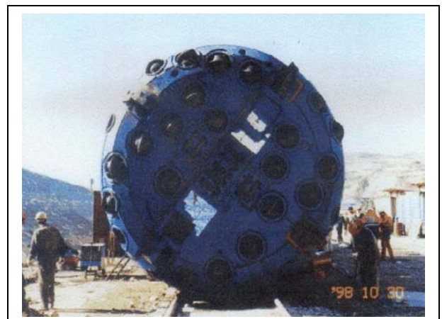
Figure 3. View to the boring head of one of DS-TBMs.
