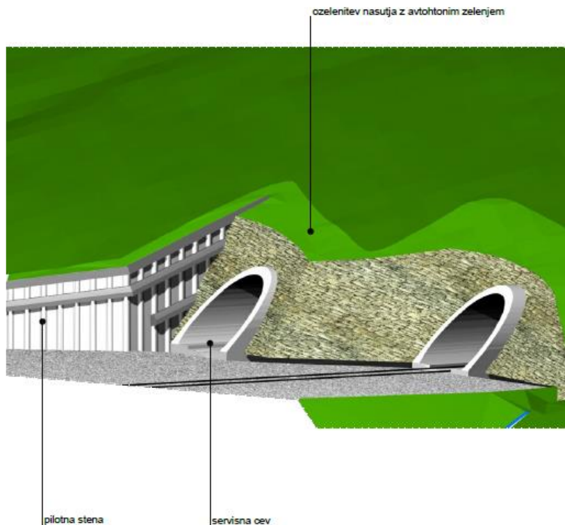
Figure 3: View to the North portal of the tunnel T8 with single track active and service tunnel without track structure.
