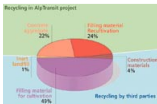
Fig. 18: Gotthard base tunnel, recycling of excavated material.
