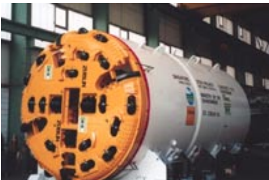
Figure 4: EPB TBM for Contract T-06.
