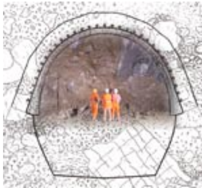
Fig. 13: Tunnel Bodio, tunnel section in loose rock material.
