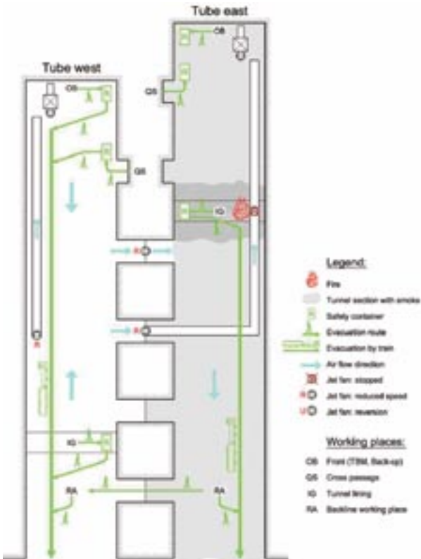
Fig. 9: Fire event with blocked staff at the front
